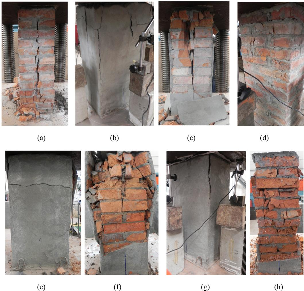
**Fig. 5.** Failure modes: (a) unconfined; (b) M-U-C; (c) crushing of slender prisms; (d) M-H-U; (e) M-U-H; (f) severely crushing of masonry; (g) M-H-H; (h) moderately crushing of masonry.
